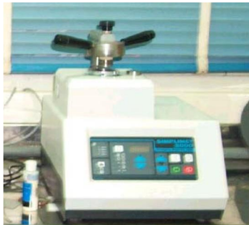
Fig. 1: A Hot Mounting Press
